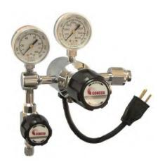
The 308 Series regulators are specifically designed to prevent freezing problems associated with high flows of carbon dioxide and nitrous oxide. As carbon dioxide or nitrous oxide passes through a regulator seat dry ice can form if the flow is too high causing the regulator to freeze up. Heating the regulator increases the flow capacity.
